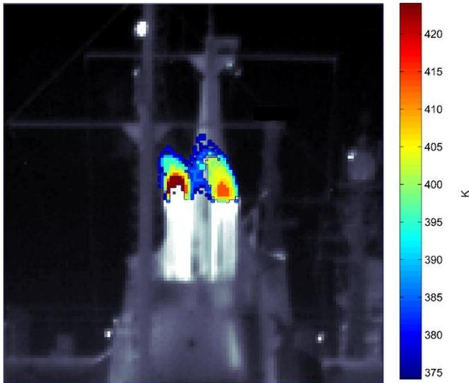
Figure 4 Gas plume temperature map associated with a single datacube of the imaging sequence derived from radiative transfer model presented in Equation 1. Temperature results are displayed over the associated broadband infrared image for clarity purposes.
