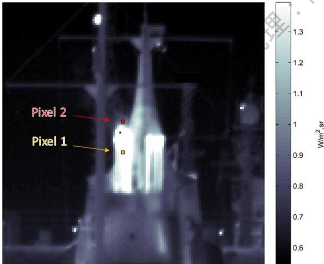
Figure 2 Broadband infrared image of a ship plume. Selected pixels are labeled for further discussion.
