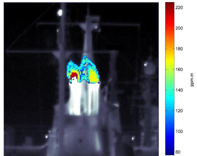
Figure 6 Carbon monoxide (CO) column density map associated with a single datacube of the imaging sequence. Results are displayed over the associated broadband infrared image for clarity purposes.
