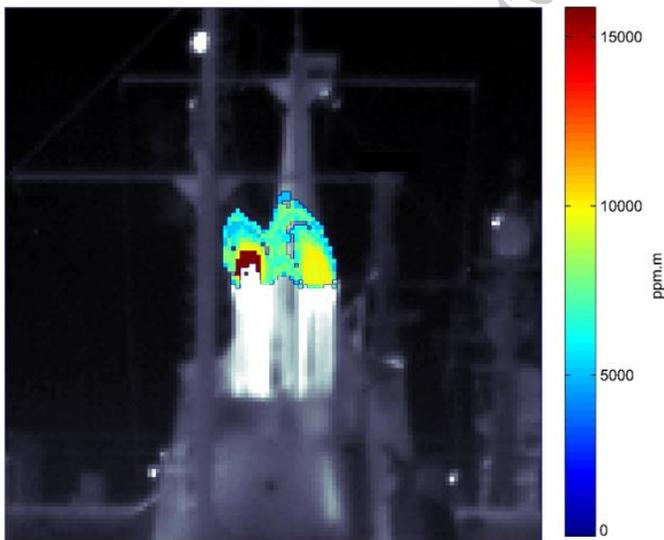
Figure 5 Carbon dioxide (CO<sub>2</sub>) column density map associated with a single datacube of the imaging sequence. Results are displayed over the associated broadband infrared image for clarity purposes.
