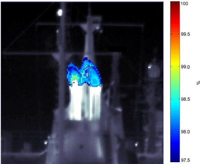
Figure 7 Combustion efficiency map associated with a single datacube of the imaging sequence. Results are displayed over the associated broadband infrared image for clarity purposes.
